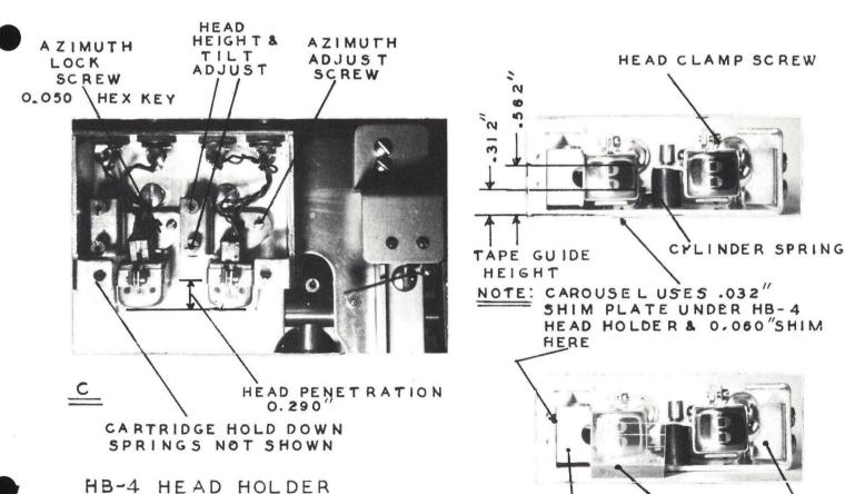
NOTE: CAROUSEL USES .032" SHIM PLATE UNDER HB-4 HEAD HOLDER & 0,060 "SHIM TAPE GUIDE GUIDE HEAD GAGE
